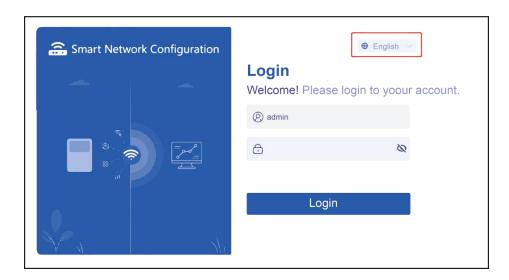
Note: When WLan-WW dataloger is used for the first time, enter the initial password, click login, the page jumps to the change password page (as below), you need to change the login password. When you change the login password, the WIFI password is also changed.
