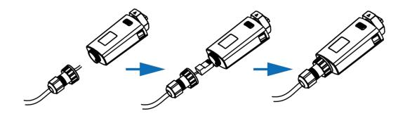
Rotate the nut at the top of the WLan-WW to make sure the triangle logo is centered on the front. Plug the WLan-WW into the "WIFI/4G/USB" port at the bottom of the inverter. Tighten the nut clockwise as follows.
