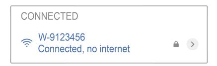
2) After connecting successfully. Open browser and enter 'https://192.168.1.1' on the address bar on top.
