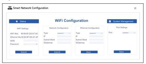
Tip: You can check the "Status" page, if it shows "Enter transparent mode", it means the network has been successfully configured.
